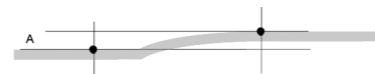
Deformation value is the height difference A between the two points shown.
